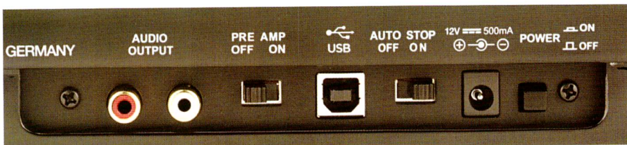
The rear panel with analogue phono output, preamp switch, USB B connector and 12V d.c. input from an external supply.
